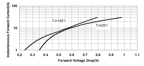
Fig.3-Typical Forward Voltage Drop Characteristics
